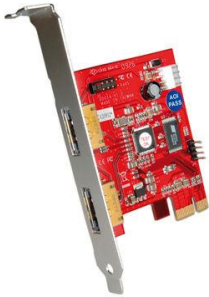
Adaptador PCI-Express 2 x eSATAp + USB - AVD. PCI-Express Adapter, 2 x eSATAp+USB -AVD.
