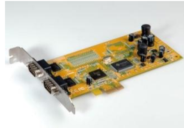
Adaptador PCI-Express 2 x RS232 - AVD. PCI-Express Adapter, 2 x RS232 Ports - AVD.
